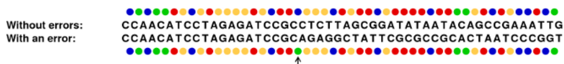
Figure 5.19: How an error in color space leads to a phase shift and subsequent problems for the rest of the read sequence
